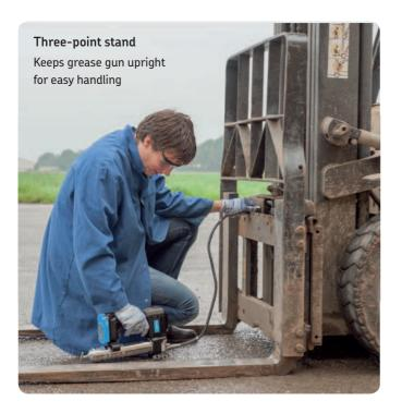
The tool's display indicates battery charge level, amount of grease dispensed, pump/motor speed and blocked lubrication points. This versatile grease gun provides two flow rates – low and high – and can dispense up to 15 grease cartridges per battery charge. The TLGB 20 can deliver pressures up to 700 bar (10 000 psi) and features a built-in light to illuminate the work area.
